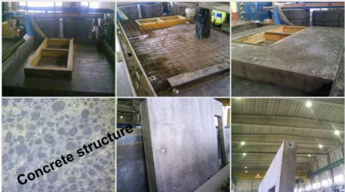
7 - Production of panels 20cm thick of (II.) Self-compacting concrete with a density of 1980kg/m 3 containing
