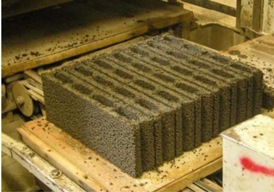
Partition block production with lightweight artificial aggregate (by ADLER device)
