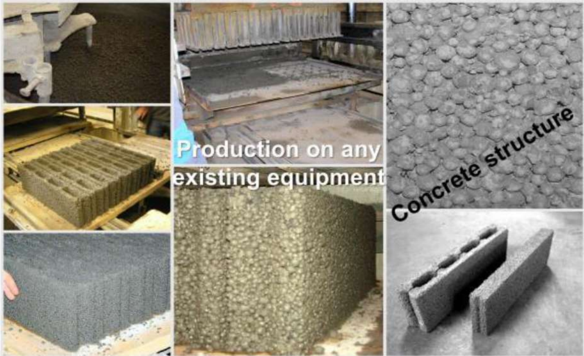
8 Production of Masonry blocks with a bulk density from 900\text{kg/m}^3
